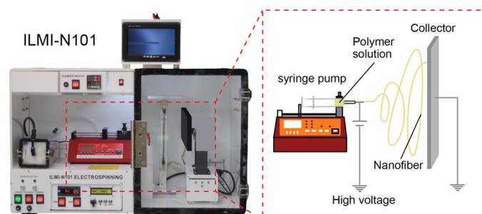
**Figure 1.** ILMI-N101 electrospinning device and its schematic illustration
