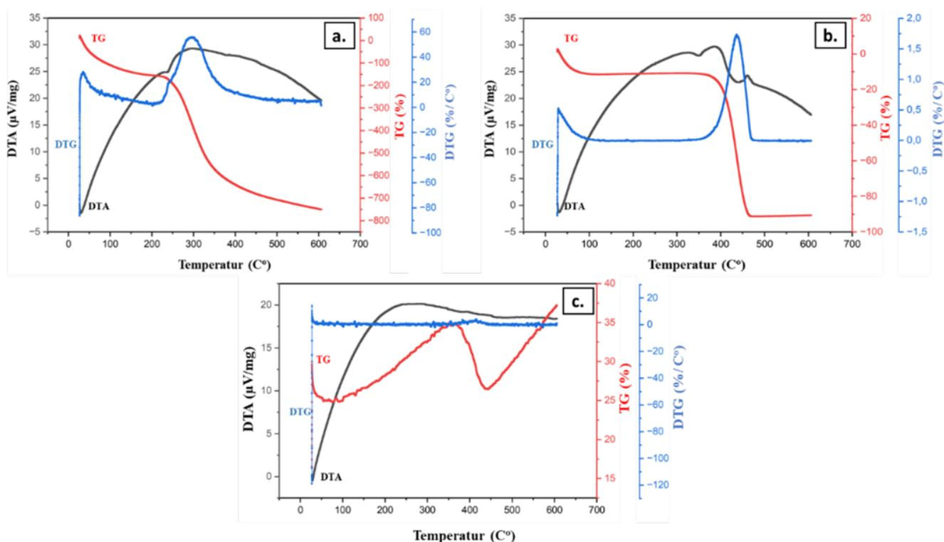
**Figure 7.** Thermal graphs of TG, DTG, and DTA for (a) pure EBN, (b) PVP powder, and (c) EBN/PVP nanofiber.
