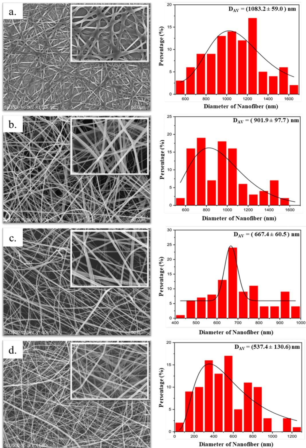
**Figure 2.** SEM images of EBN/PVP nanofibers and their corresponding diameter distributions at various voltages of (a) 10 kV, (b) 12.5 kV, (c) 15 kV and (d) 17.5 kV.
