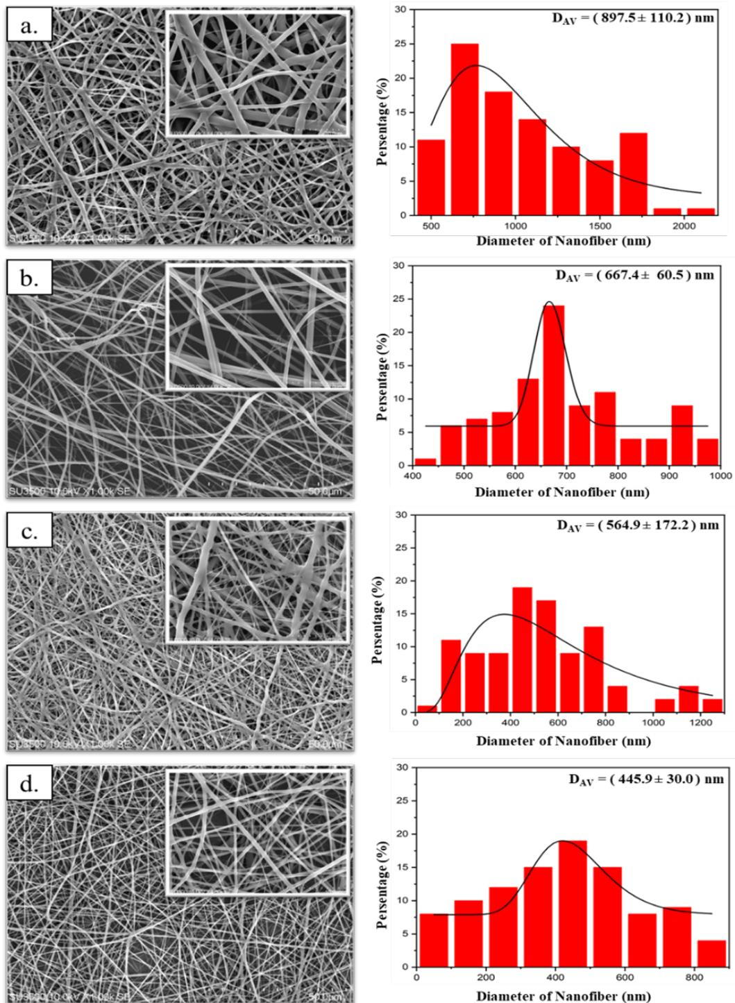
**Figure 4.** SEM images of EBN/PVP nanofibers and their corresponding diameter distributions fabricated using various collector distances of (a) 18 cm, (b) 20 cm, (c) 22 cm, (d) 24 cm.
