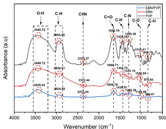
**Figure 6.** FTIR plots for EBN, PVP, and EBN/PVP (60:40) samples.
