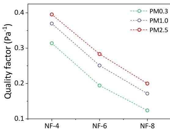
**Figure 5.** The quality factor of fabricated nanofiber as PM filtration membrane
