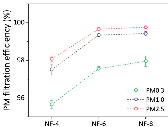
**Figure 6.** The recap of fabricated PM filtration membrane efficiency towards PM0.3, PM1.0, and PM2.5.
