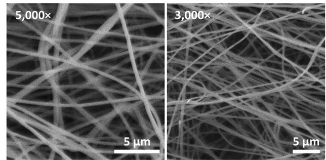
**Figure 2.** Scanning electron microscopy (SEM) images of fabricated PAN nanofiber with different magnification of 5,000× and 3,000×
