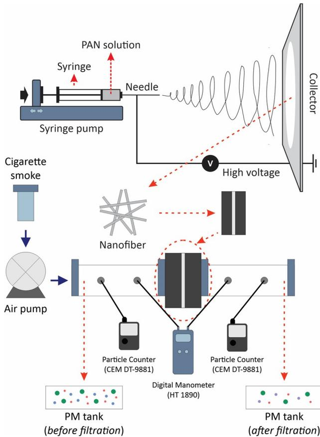
**Figure 1.** Nanofiber fabrication process using electrospinning method and PM filtration testing setup
