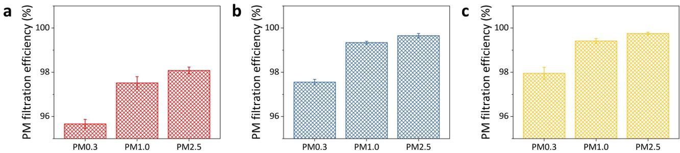
**Figure 4.** The filtration efficiency of PM0.3, PM1.0, and PM2.5 of (a) NF-4, (b) NF-6, and (c) NF-8 membranes
