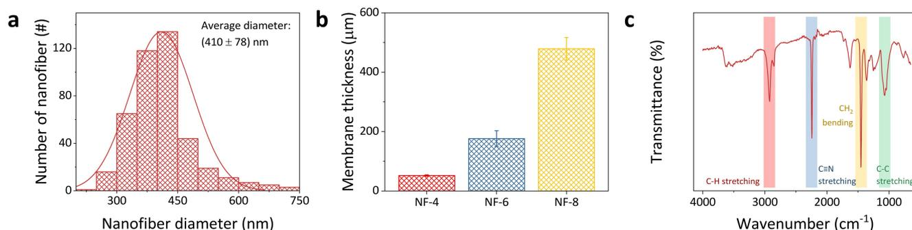
**Figure 3.** (a) Diameter distribution of fabricated PAN nanofiber. (b) The thickness of nanofiber-based PM filtration membrane with various solution volumes of 4 mL, 6 mL, and 8 mL (denoted as NF-4, NF-6, and NF-8, respectively). (c) Fourier-transform infrared spectroscopy of fabricated PAN nanofiber.
